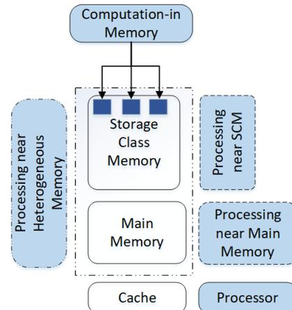
**Fig. 2: Processing options in the memory hierarchy**
