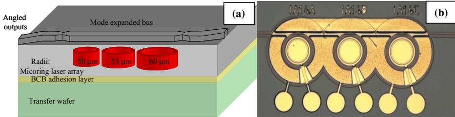
Fig. 1. (a) Schematic diagram for the bus coupled microring laser array showing micro-rings with three distinct radii and the mode expanded bus design. The  $60\mu\text{m}$  and  $55\mu\text{m}$  radius rings emit at  $1561\text{nm}$  and  $1567\text{nm}$  respectively (b) Photograph of the microring laser array
