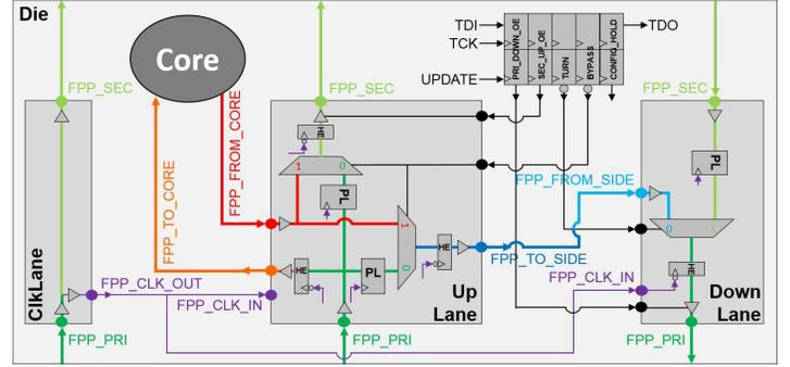
Figure 4: FPP example following the Test@First FPP architecture.
