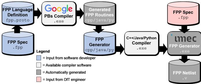
Figure 2: Flow for the definition of an FPP specification language and development of an FPP spec-to-netlist generator as demonstrator application.
