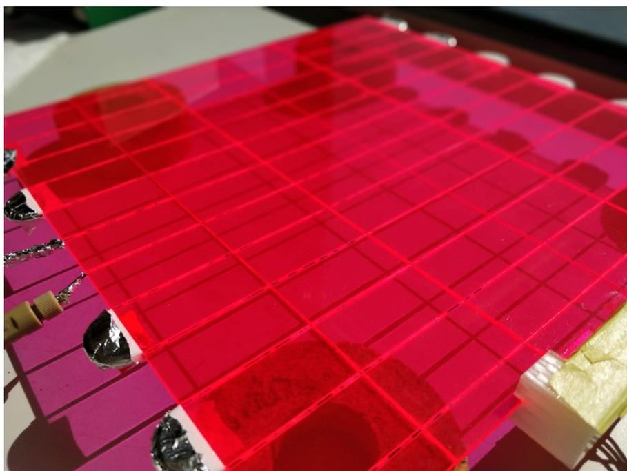
*A red LSC-PM reactor next to a window, while illuminated by sunlight. Inside the reactor channels, blue slugs containing the reaction are visible. On the right side, the light sensor.*
