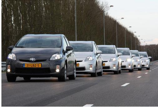
**Fig. 1.1.** Example of a NCS: Cooperative and automated driving cars driving in a platoon (Courtesy of the Dutch Institute for Applied Scientific Research (TNO)).
