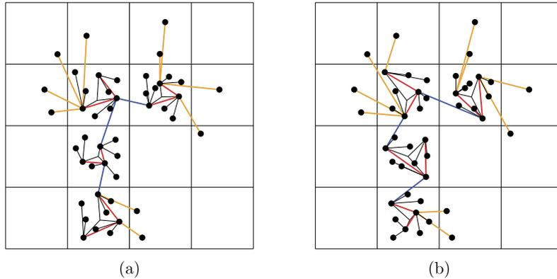
**Fig. 13.** The distributed approach: a grid is placed over the point set and different representatives construct different graphs ((a) and (b)). The red and black edges form the tree in each dense cell, blue edges connect the dense cells, and orange edges connect the vertices in sparse cells.
