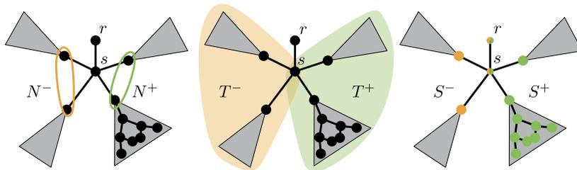
Fig. 5. Illustration of the various definitions used in Section 2.2. Grey triangles illustrate further subtrees, one shows interior vertices purely for illustrative purposes.
