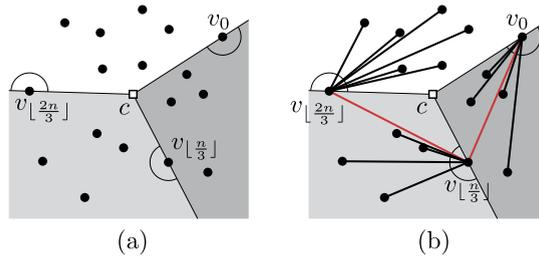
**Fig. 12.** Extracting one layer: (a) The three sectors defined by  $v_0$ ,  $v_{\lfloor \frac{2n}{3} \rfloor}$ , and  $v_{\lfloor \frac{n}{3} \rfloor}$ . (b) Connecting the points to the representative of their sector. The red edges connect the representatives.
