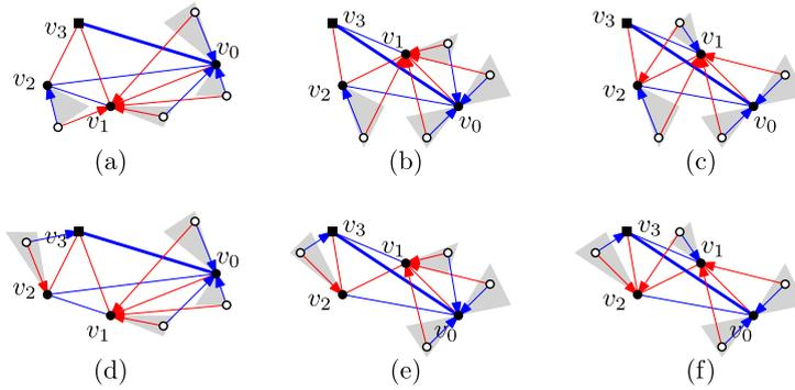
**Fig. 9.** The different plane spanning trees  $R$  and  $B$  for case 1 when  $P$  is in convex position. The bold blue edges  $v_3v_0$  are edges of  $MST^3(S)$ , i.e., edges with link distance 3 in  $MST(S)$ , that might still be crossed. Note that  $v_3v_0$  can only be crossed in Cases (a) and (b), as in the other cases this edge is surrounded by “uncrossable”  $MST^2(S)$ -edges.
