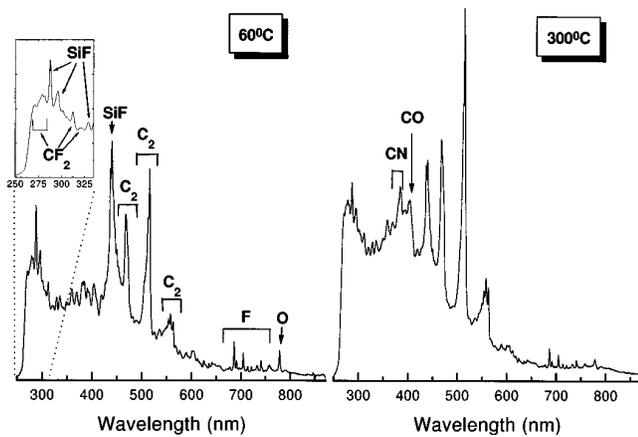
FIG. 7. Comparison of optical emission spectra measured on a  $C_3F_6$  plasma at 1400 W inductive power and 6 mTorr operating pressure. The left panel shows the spectrum measured in a cold (60 °C) reactor and the right panel shows the spectrum measured in a hot (300 °C) reactor.
