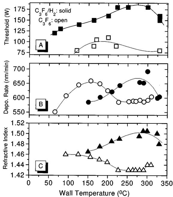
FIG. 10. (A) Threshold RF bias power for etching, (B) passive fluorocarbon deposition rate, and (C) the fluorocarbon refractive index as a function of reactor wall temperature in a C<sub>3</sub>F<sub>6</sub> (40 sccm) and a C<sub>3</sub>F<sub>6</sub>/H<sub>2</sub> (40 sccm/12 sccm) plasma at 1400 W inductive power and 6 mTorr operating pressure.
