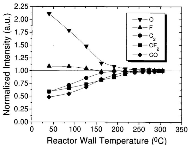
FIG. 8. Emission intensities measured in a  $C_3F_6$  plasma at 1400 W inductive power and 6 mTorr operating pressure. The intensities of the various species are normalized to their value in a hot reactor.
