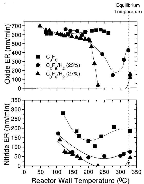
FIG. 11. (A) Oxide etch rates and (B) nitride etch rates as functions of wall temperature measured in C<sub>3</sub>F<sub>6</sub> (40 sccm), C<sub>3</sub>F<sub>6</sub>/H<sub>2</sub> (40 sccm/12 sccm), and C<sub>3</sub>F<sub>6</sub>/H<sub>2</sub> (40 sccm/15 sccm) discharges at 1400 W inductive power and 6 mTorr operating pressure at a RF bias power of 200 W (i.e., -100 V self-bias).
