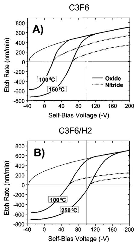
FIG. 12. Schematic view of the oxide and nitride etch characteristics for various wall temperatures for (A)  $C_3F_6$  processing and (B)  $C_3F_6/H_2$  processing. The thick solid curves represent the oxide etching, and the dotted lines the nitride etching. The sputtering curve (thin solid line) is also included.
