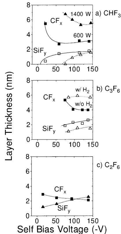
FIG. 4. Steady state CF<sub>x</sub> (closed symbols) and SiF<sub>y</sub> (open symbols) layer thicknesses as a function of the self-bias voltage for different fluorocarbon plasmas: (a) 40 sccm CHF<sub>3</sub>, 6 mTorr, for two inductive powers: squares 600 W, triangles 1400 W; (b) 20 sccm C<sub>3</sub>F<sub>6</sub>, 6 mTorr, 1400 W, with hydrogen addition: squares 0 sccm H<sub>2</sub>, triangles 12 sccm H<sub>2</sub>; (c) 40 sccm C<sub>2</sub>F<sub>6</sub>, 6 mTorr, 1400 W.
