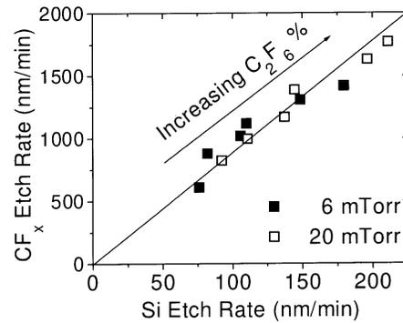
FIG. 3. Fluorocarbon etch rate vs silicon etch rate for two different operating pressures. The flow ratio of C<sub>2</sub>F<sub>6</sub> and C<sub>3</sub>F<sub>6</sub> was changed in steps of 20% while the self-bias voltage, pressure, and the inductive power were fixed at -85 V, 6 mTorr, and 1400 W, respectively.
