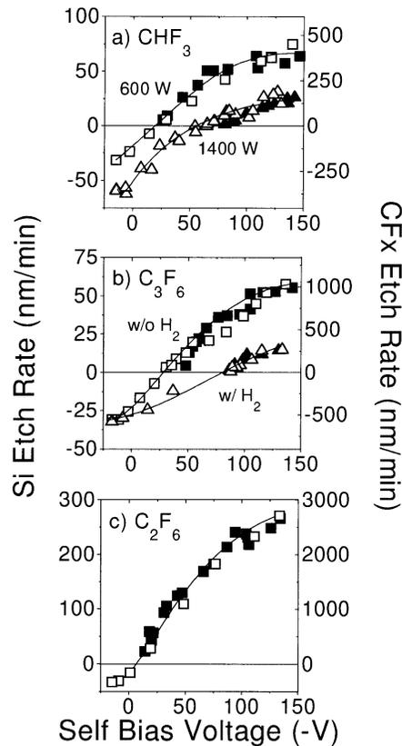
FIG. 2. Silicon (closed symbols) and fluorocarbon (open symbols) etch rates as a function of self-bias voltage for different fluorocarbon plasmas: (a) 40 sccm CHF<sub>3</sub>, 6 mTorr, for two inductive powers: squares 600 W, triangles 1400 W; (b) 20 sccm C<sub>3</sub>F<sub>6</sub>, 6 mTorr, 1400 W, with hydrogen addition: squares 0 sccm H<sub>2</sub>; triangles 12 sccm H<sub>2</sub> (c) 40 sccm C<sub>2</sub>F<sub>6</sub>, 6 mTorr, 1400 W.
