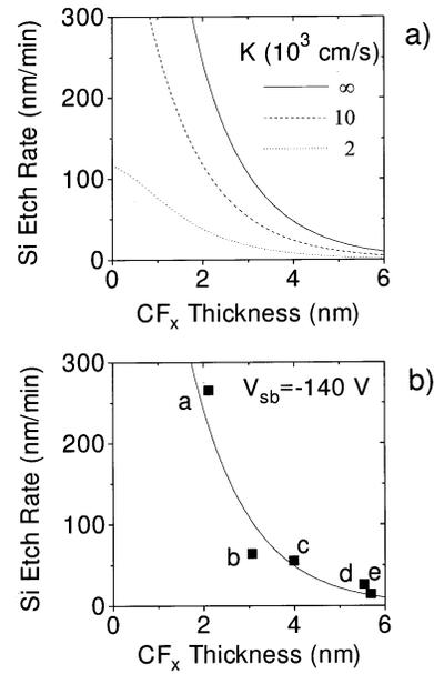
FIG. 9. Silicon etch rate vs  $\text{CF}_x$  layer thickness. (a) The model. (b) The experimental data in comparison with an exponential fit ( $y = A \exp(-Bx)$ ). In (b) a:  $\text{C}_2\text{F}_6$  1400 W; b:  $\text{CHF}_3$  600 W; c:  $\text{C}_3\text{F}_6$  1400 W; d:  $\text{CHF}_3$  1400 W; e:  $\text{C}_3\text{F}_6/\text{H}_2$  1400 W.
