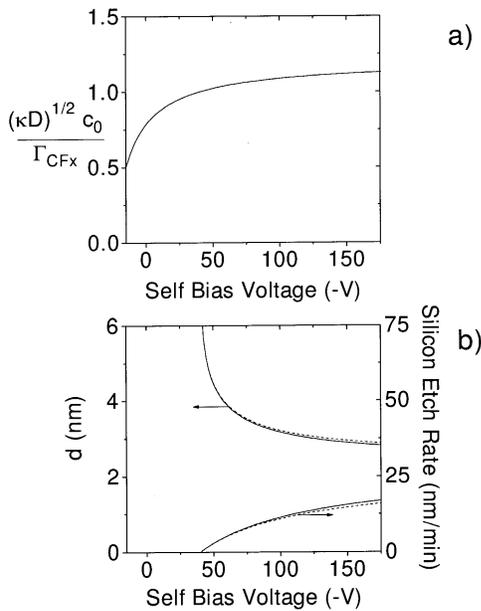
FIG. 10.  $CF_x$  layer thickness ( $d$ ) and the silicon etch rate ( $\Gamma_{Si}$ ) as a function of the self-bias voltage according to the model presented. In (a) the input that is used, which can be explained by an enhancement in the diffusion transport or by ion impact fragmentation and surface dissociation is shown. The solid lines in (b) represent the numerical solutions of Eqs. (3), (8), and (9). The dashed lines represent the analytical solutions given by Eqs. (12) and (13).
