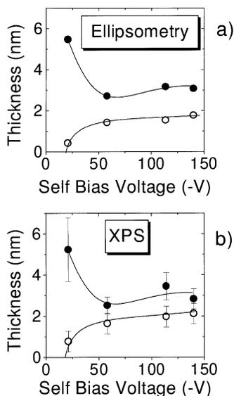
FIG. 7. CF<sub>x</sub> and SiF<sub>y</sub> layer thicknesses determined by (a) ellipsometry and (b) XPS. The samples analyzed were processed in a 40 sccm CHF<sub>3</sub> discharge at 6 mTorr and maintained by 600 W inductive power.
