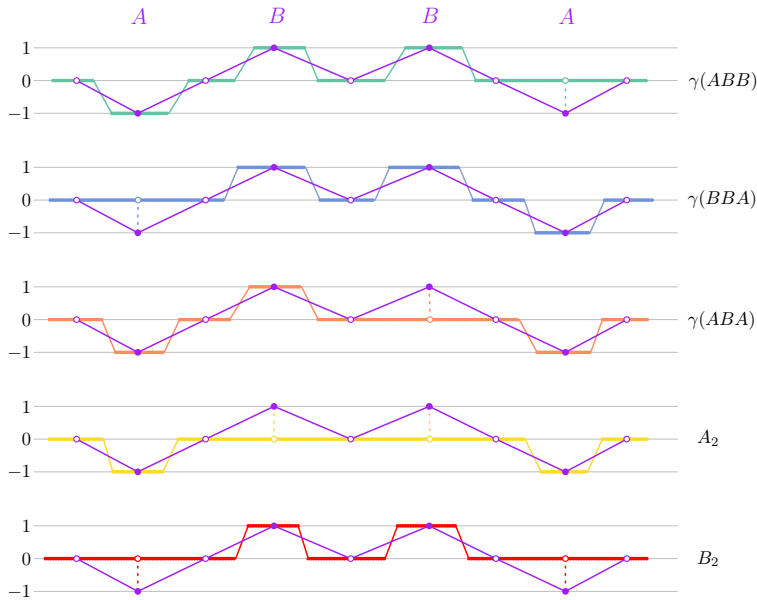
■ Figure 2 Five curves from G \cup R_{i,j} in the reduction for the DTW average curve problem and a center curve constructed from the string ABBA (purple) as in Lemma 5. Fat horizontal lines indicate \beta consecutive vertices. Vertices that match at distance 0 touch, vertices that match at distance 1 are indicated by dotted lines. The center has 1 mismatch with the first 3 curves and 2 with the final two, so the total cost here is 3 \cdot (1^p)^{q/p} + 2\alpha \cdot (2 \cdot 1^p)^{q/p} = 3 + 2\alpha \cdot 2^q
