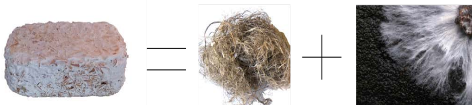
Fig. 1; A mycelium-based material is a composite consisting of a natural reinforcement or filler, such as hemp fibers, and the mycelium of a fungus.
