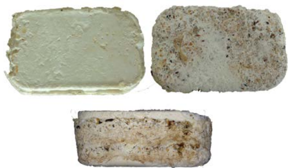
Fig. 3 ; from top left, going clockwise: top, bottom and side view of a sample of C. Versicolor and non-woven hemp mats.
