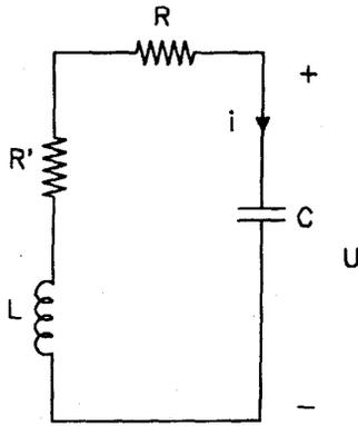
Fig. 3. Replacement circuit for the grid oscillator.
