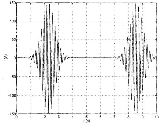
Fig. 5. Oscillator current  $i$  for  $p = 0.1592$  Hz. The plot is calculated from (28).
