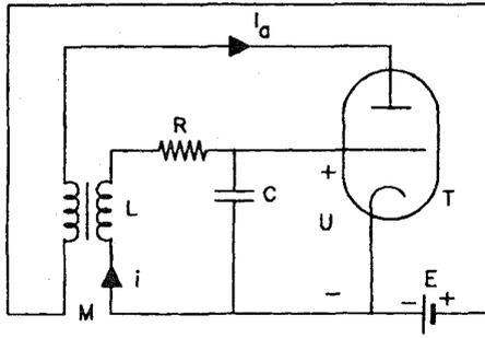
Fig. 2. Grid oscillator.
