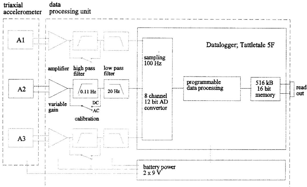
Fig. 5. Block-diagram of the TA and the data unit for acquisition, processing and storage of accelerometer output. The complete data processing is indicated for one of the uniaxial accelerometers ( $A_2$ ).
