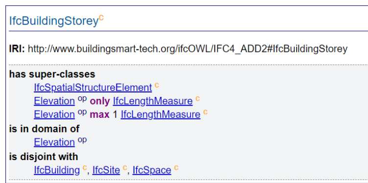
Figure 1 The definition for ifcBuildingStorey in the ifcOWL ontology (Pauwels & Terkaj 2015)
