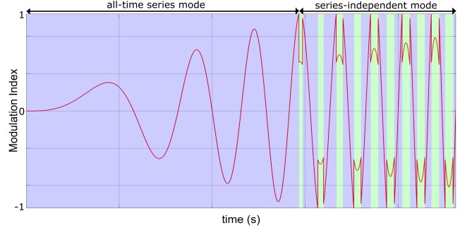
Figure 3: Winding Reconfiguration Based on Modulation Index (Independent Mode is Marked with Green Area).
