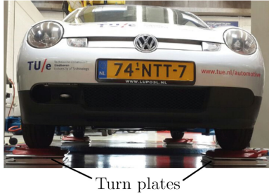
Fig. 8. Test vehicle in the laboratory with the wheels on quasi frictionless turn-plates.
