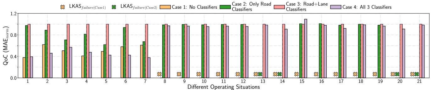
Fig. 6. Analysis of LKAS robustness and performance for different static situations. Four different cases are considered by incremental addition of classifiers. Lower MAE implies better LKAS performance. All values are normalized to case 3. Situations 1-21 are defined in Table. III.
