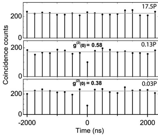
FIG. 3. Coincidence counts as a function of delay at various pump powers ( $P$  corresponds the saturation power of the exciton) on the X line of a QD having similar spectral features as the QD shown in Figs. 1 and 2.
