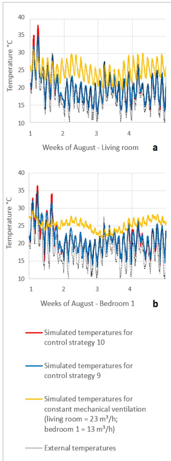
Figure 6: External and Simulated temperatures
