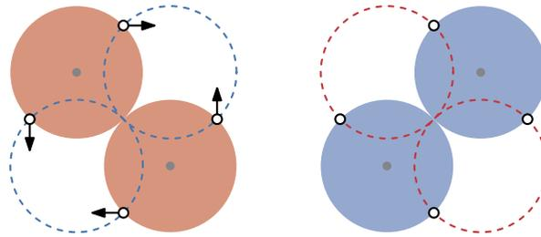
**Fig. 1.** A small change in point positions causes a large change in the smallest 2 covering disks: moving the points along the arrows changes the optimal solution from the red to the blue solution. The optimal centers are marked in grey, while sub-optimal solutions are shown as dashed circles. (For interpretation of the colors in the figure(s), the reader is referred to the web version of this article.)
