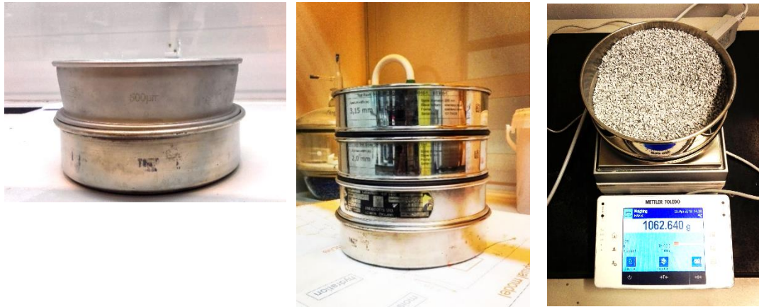
Figure 3.7: Procedure of sieving performed to investigate the particle size distribution [Left] Sieving with a sieve size of 500 \mu\text{m} to remove powder from the sample [Middle] Sieving with a stack of sieve size of 1 mm, 2 mm and 3.15 mm [Right] Total weight of the sample after sieving (including container weight)
