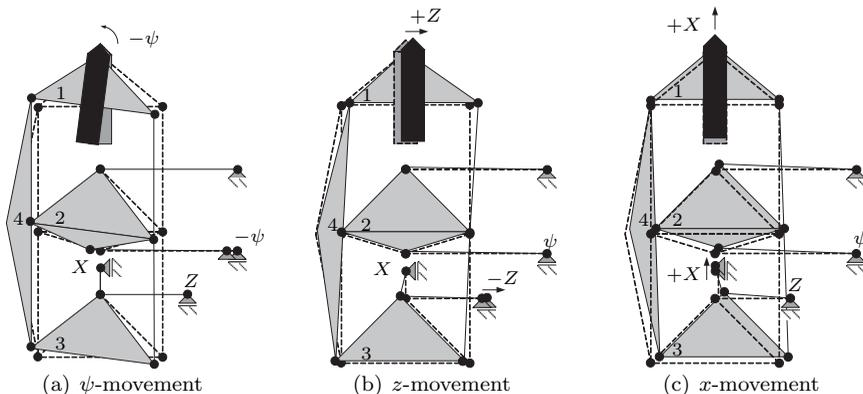
Figure 3: Positioning system's mechanism in 2d, with the tool on body 1
