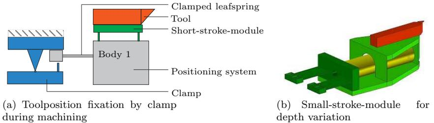
Figure 4: Toolholder's fixation clamp and short-stroke-module
