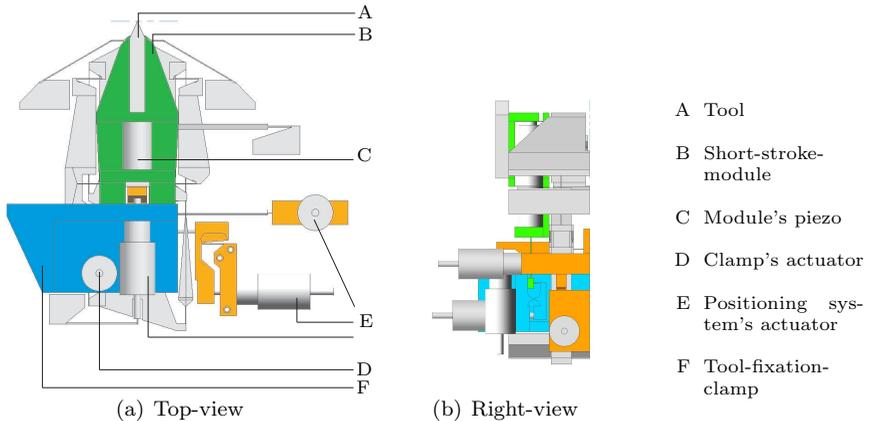
Figure 2: Toolholder for intuitive manual tool position adjustment of the profile tool. Using this toolholder reduces the maximum position adjustment time
