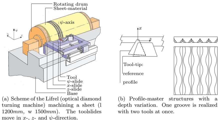
Figure 1: Lifrel and an example of an optical groove master structure
