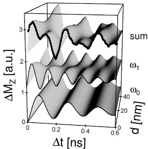
FIG. 4. Observation of standing spin waves. Because of the nonuniform heating by the pump-pulse both the fundamental precession ( $\omega_0$ ), which is uniform in the depth  $d$  of the layer, and the first-order standing spin wave ( $\omega_1$ ) are excited. From the resulting precession (sum) only the magnetization near the surface is optically measured. The measurement is thus shown at  $d = 0$  nm by solid dots.
