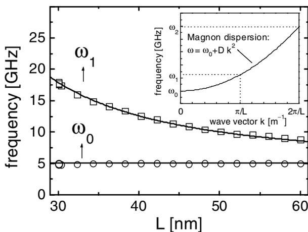
FIG. 5. Fundamental ( $\omega_0$ ) and first-order ( $\omega_1$ ) spin-wave frequency ( $\omega/2\pi$ ) in Ni versus layer thickness  $L$ . The solid lines are fits to the data. Inset: schematic magnon dispersion relation.
