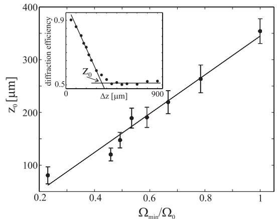
FIG. 2. Experimental verification of the scaling law  $t_0 \sim 1/\Omega_0$  connecting the characteristic time  $t_0 \equiv z_0/v$  when Michelangelo wave packets form and the Rabi frequency  $\Omega_0$ . The line is a guide to the eye. We measure the zeroth order diffraction efficiency as a function of  $\Delta z$  (inset) for different Rabi frequencies. The crossing point between the linear extrapolation of the short and long-time limits yields  $z_0$ .
