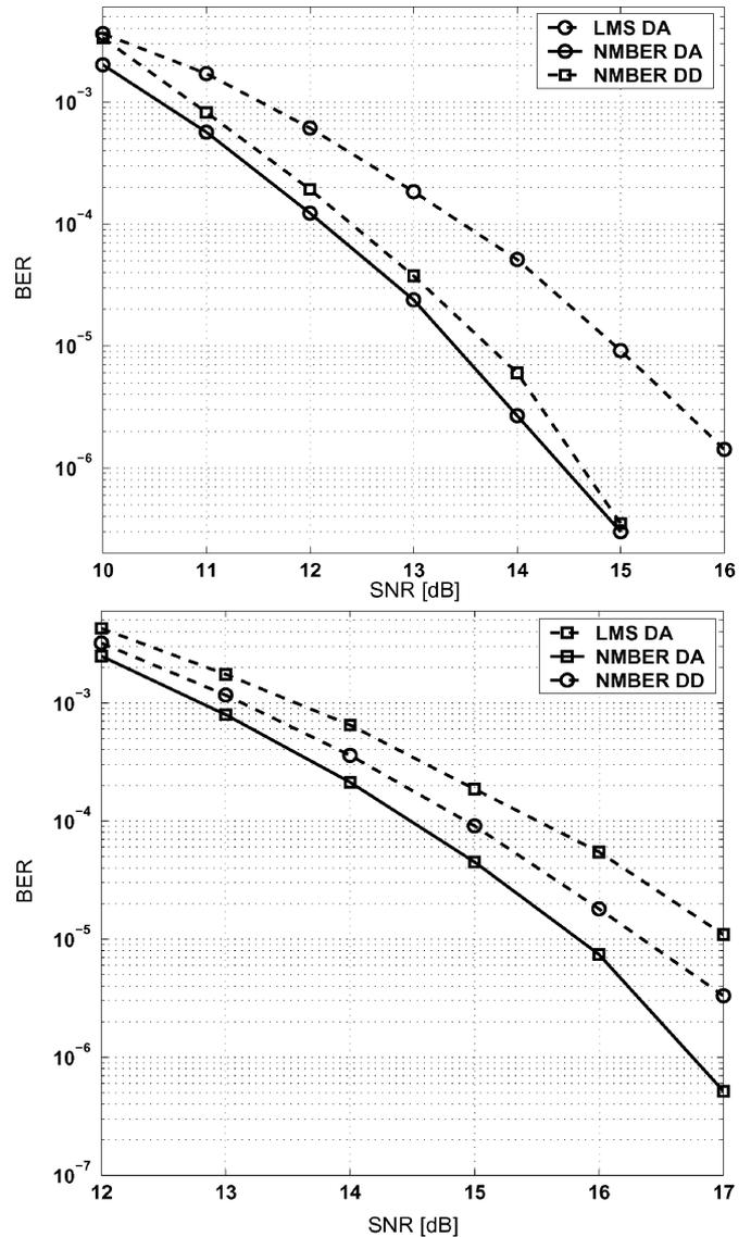
Fig. 11. Simulated BER versus SNR using the NMBER algorithm in both the DA and DD modes for  $g = g^0$  and the 23-GB channel (upper plot;  $\alpha = 0.4$ ) and for  $g = g^2$  and the 30-GB channel (lower plot;  $\alpha = 0.3$ ). As a basis of reference, the LMS performance in DA mode is also shown.
