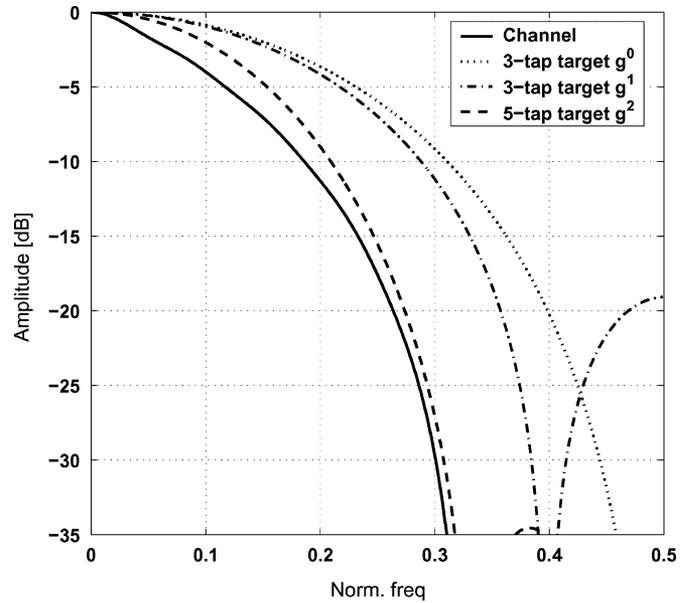
Fig. 5. Amplitude–frequency of idealized optical channel having a normalized cutoff  $f_c = 0.34$ , 3-tap targets  $g^0 = [1, 2, 1]$  and  $g^1 = [1, 1.6, 1]$  and 5-tap target  $g^2 = [0.17, 0.5, 0.67, 0.5, 0.17]$ . For clarity of the plot, the different targets are normalized to have the same DC.
