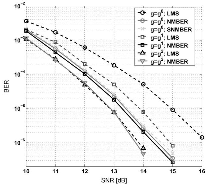
Fig. 7. Simulated BER versus SNR for the different target responses and adaptation schemes at a disk capacity of 23 GB.
