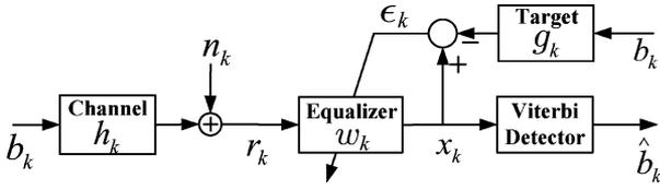
Fig. 1. Discrete-time model of a PRML system.
