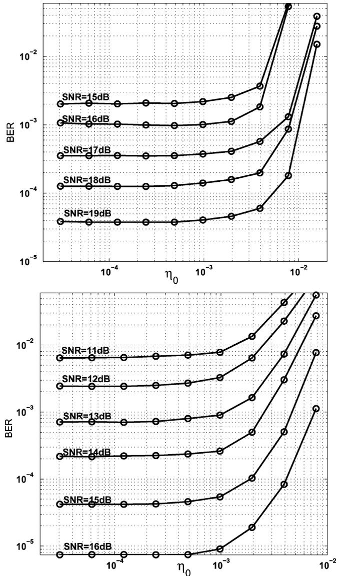
Fig. 10. Simulated BER versus  $\eta_0$  at a capacity of 30 GB and different SNR values for the target responses  $g = g^0$  (upper plot) and  $g = g^2$  (lower plot).
