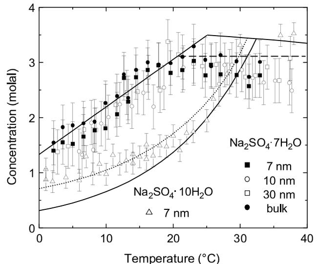
FIG. 4. Measured solubility of  $\text{Na}_2\text{SO}_4$  in bulk and inside the pores of various Nucleosils. The horizontal dashed line represents the solubility at 60 °C. Solid lines and curves reflect bulk solubilities. The dotted curve through the data indicating the presence of  $\text{Na}_2\text{SO}_4 \cdot 10\text{H}_2\text{O}$  in the 7 nm pores is meant only as a guide to the eye.
