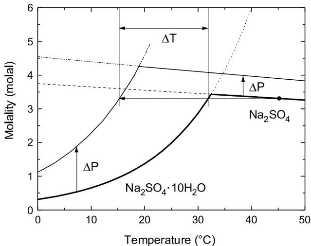
FIG. 2. An illustration of the change of the solubility and the temperature shift  $\Delta T$  of the phase transformation of  $\text{Na}_2\text{SO}_4$  when a pressure  $\Delta p$  is applied. The curves are calculated from Eq. (2).
