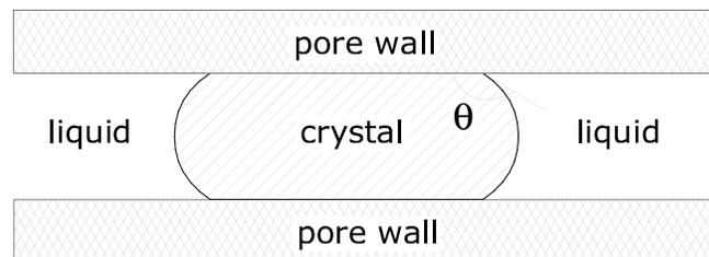
FIG. 1. Crystal confined in a cylindrical pore.
