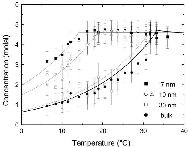
FIG. 3. Solubility of  $\text{Na}_2\text{CO}_3$  in bulk and inside the pores of various Nucleosils. The curves reflect the bulk literature values or a description of the data by Eq. (2). For the 10 nm pores, measurements were performed on two different Nucleosil samples.
