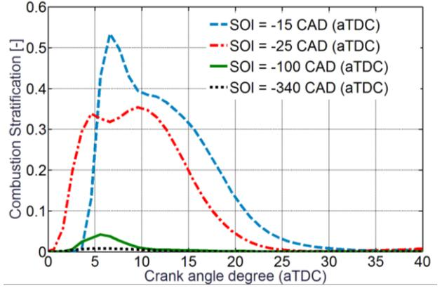
Fig. 5. Time resolved combustion stratification for different injection timings.
