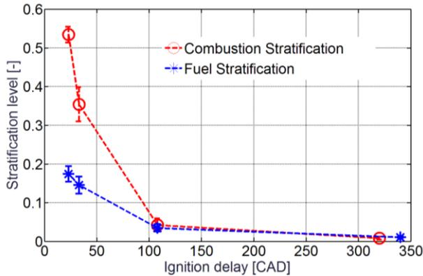
Fig. 7. Fuel and combustion stratification versus ignition delay.
