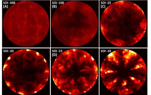
Fig. 6. Fuel distributions for different injection timings.
