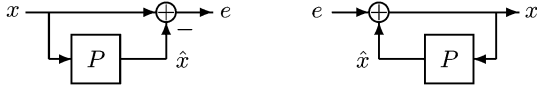
Fig. 4. Analysis and synthesis filter realization with the predictor P in a feed-forward and feedback loop, respectively.
