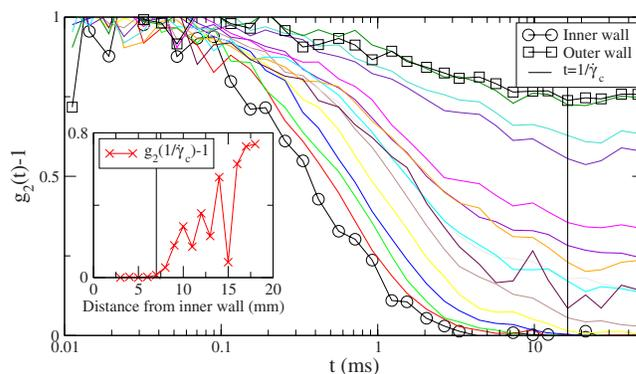
FIG. 5. (Color online) DWS time correlation measurements of the fluid inside and outside the sheared band in a Couette geometry. The inset shows the correlation function at  $t=1/\dot{\gamma}_c$  (which is a characteristic relaxation time of the material) as function of the distance from the inner wall. The tendency for much longer correlation times in the solid phase as compared to the sheared phase is very clear, and similar to a simulation of a model glass that exhibits shear banding [2].
