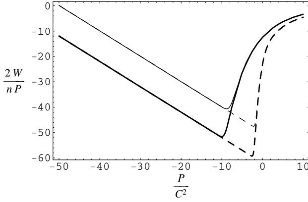
Fig. 2. The relative error due to clipping and quantization according to (10) (in dB) as a function of  $P/C^2$  (in dB) for  $n = 2N_c = 128$  and ( $L = 256, m = 0$ ) (thin line), ( $L = 1024, m = 0$ ) (thick line), ( $L = 256, m = 20$ ) (thin dashed line) and ( $L = 1024, m = 20$ ) (thick dashed line).
