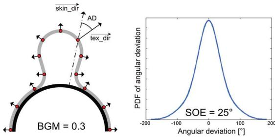
Fig. 3. Left: Illustration of arm cross sections with a potential wrinkle configuration in casual garment with  $BGM = 0.3$ . Red dots represent potential sensor locations and their normal vectors. Right: Normal vectors of skin and garment describe an AD, quantified in a distribution plot. The SOE is  $25^\circ$ . See Section IV for details.
