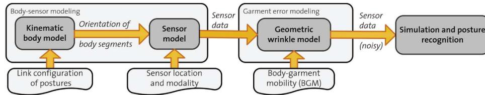
Fig. 1. Outline of our simulation framework: 1) kinematic body model using parametric descriptions of postures to derive body-segment orientation; 2) sensor model to simulate sensor readings of arbitrary inertial modalities; 3) geometric wrinkle model to estimate SOEs, as they occur in worn garments; and 4) recognition simulation to estimate the influence of orientation errors on posture discrimination.
