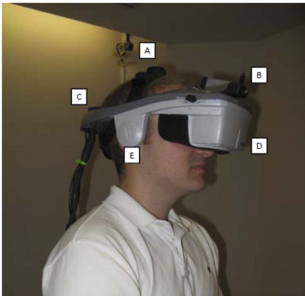
Fig. 1. The setup of the IVE used in the study. Cameras in the corners (A) of the room track the location of an infrared light (B). Accelerometers (C) located at the back of the HMD track the yaw, pitch, and roll of the head. This information is processed by a computer that renders the virtual image on the stereoscopic display of the HMD (D) and the sound through the headphones (E).
