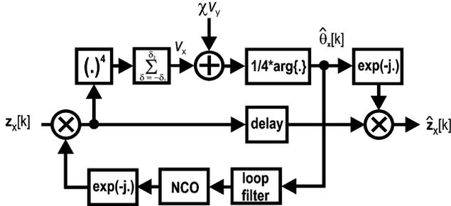
Fig. 15. Block diagram of the JP carrier phase estimator for the  $x$ -polarization with CMA equalization.
