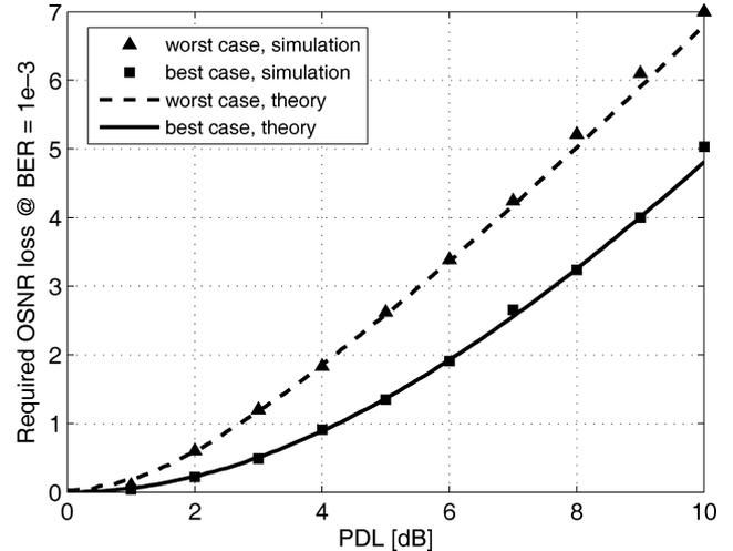
Fig. 13. Required OSNR penalty versus PDL, at 1000-ps/nm CD, 30-ps mean DGD (full-order PMD), and 15 taps of a T/2-spaced butterfly FIR and 112-Gb/s PolMux-QPSK.
