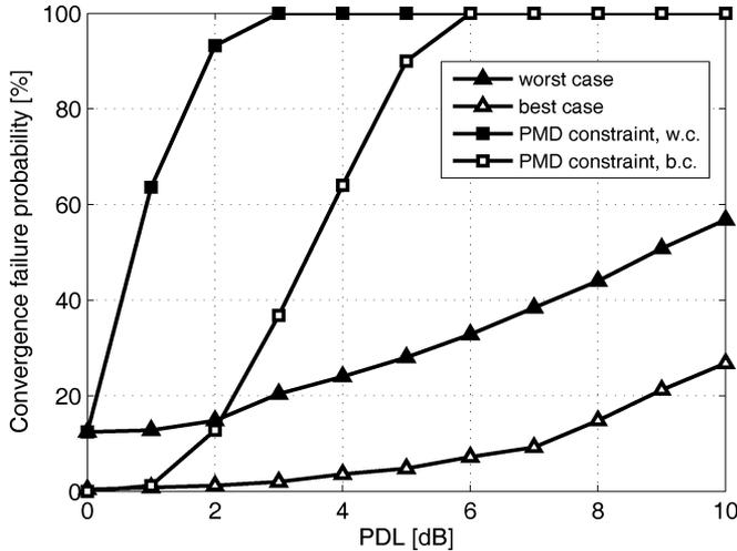
Fig. 12. Comparison of the equalizer failure probability with a degenerate solution for pure CMA/LMS and with an added constraint of a unitary PMD matrix versus PDL for 112-Gb/s PolMux-QPSK, CD = 1000 ps/nm and OSNR = 14 dB. A 15-tap T/2 filter is used for equalization.
