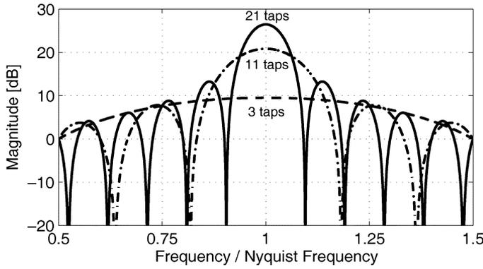
Fig. 10. Absolute value of the prefilter transfer function  $H_{\text{pre},m}$  for several filter lengths  $N_{\text{filt}}^*$ .
