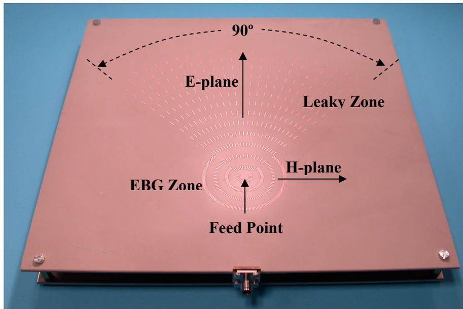
Figure 1: Antenna structure.
