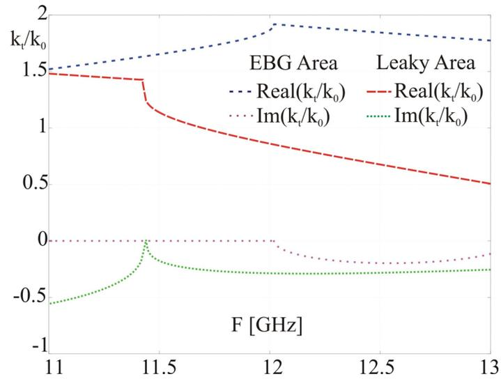
Figure3: Dispersion diagrams of the leaky and EBG zones.
