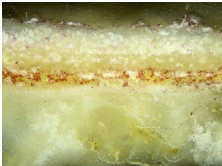
**Figure 5.** Hardham Church, West Sussex, England: Photomicrograph (200x magnification) of cross section taken from nave south side, after histochemical test for sulphate. Gypsum (identified by areas stained purple) is present solely within a yellow layer of wax (dated to 1934) between the original plaster and a surface limewash dated to 1935. (photo: A. Heritage, Conservation of Wall Painting Department, Courtauld Institute, 1994)
