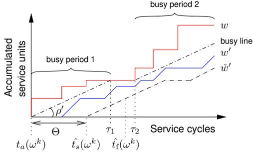
Fig. 4. Example service curves in a  $\mathcal{LR}$  server.
