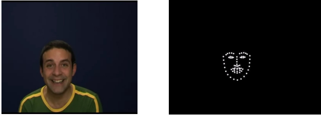
Fig. 1. An example of a frame of a full-face video and a frame of a facial-landmark video
