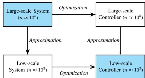
Fig. 1. Strategies for controller design for large-scale systems.
