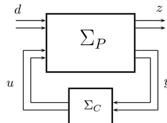
Fig. 2. Interconnection structure used in disturbance decoupling problems.
