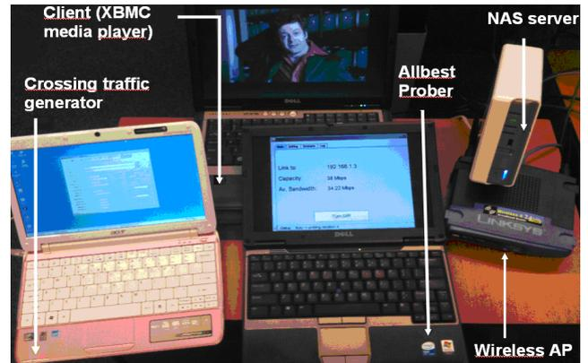
Figure 1. Our Allbest demonstrator. The probe generator runs on the Allbest Prober laptop. The crossing traffic generator is a netbook running D-ITG. Path capacity and available bandwidth estimation are shown on the GUI of the prober, while a video is being streamed from the NAS server to the XBMC media player on the client.
