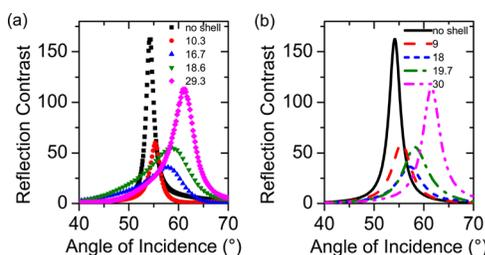
FIG. 2. (Color online) Measured reflection contrast as a function of the angle of incidence of a sample of GaP nanowires, and of similar samples in which the nanowires have been coated with  $\text{SiO}_2$  shells. (b) Fits to the measurements.
