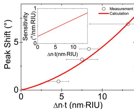
FIG. 3. (Color online) Measured and calculated shift of the peak in reflection contrast as a function of the product of the SiO<sub>2</sub> thickness,  $t$ , and the difference in refractive index  $\Delta n$ , between the shell and the surrounding medium. The inset shows the sensitivity of the shift as a function of  $\Delta n \cdot t$ .
