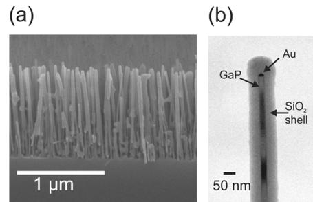
FIG. 1. (a) Cross-sectional SEM image of a sample of GaP nanowires. (b) TEM image of a nanowire covered with a thin shell of SiO<sub>2</sub>.
