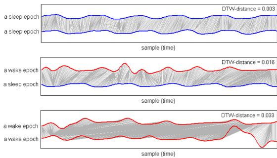
Fig. 2. Examples of two series (30 seconds each) and the alignment between them in the three situations (*upper*: two sleep epochs, *middle*: a wake and a sleep epoch, *lower*: two wake epochs) during warping process. The values of their DTW-distances are indicated.
