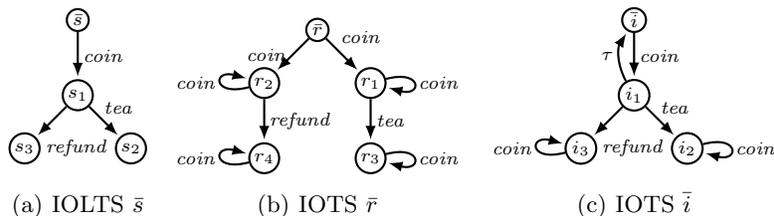
**Fig. 1.** A specification  $\bar{s}$  of a tea vending machine, a correct implementation  $\bar{r}$  and an incorrect implementation  $\bar{i}$ .
