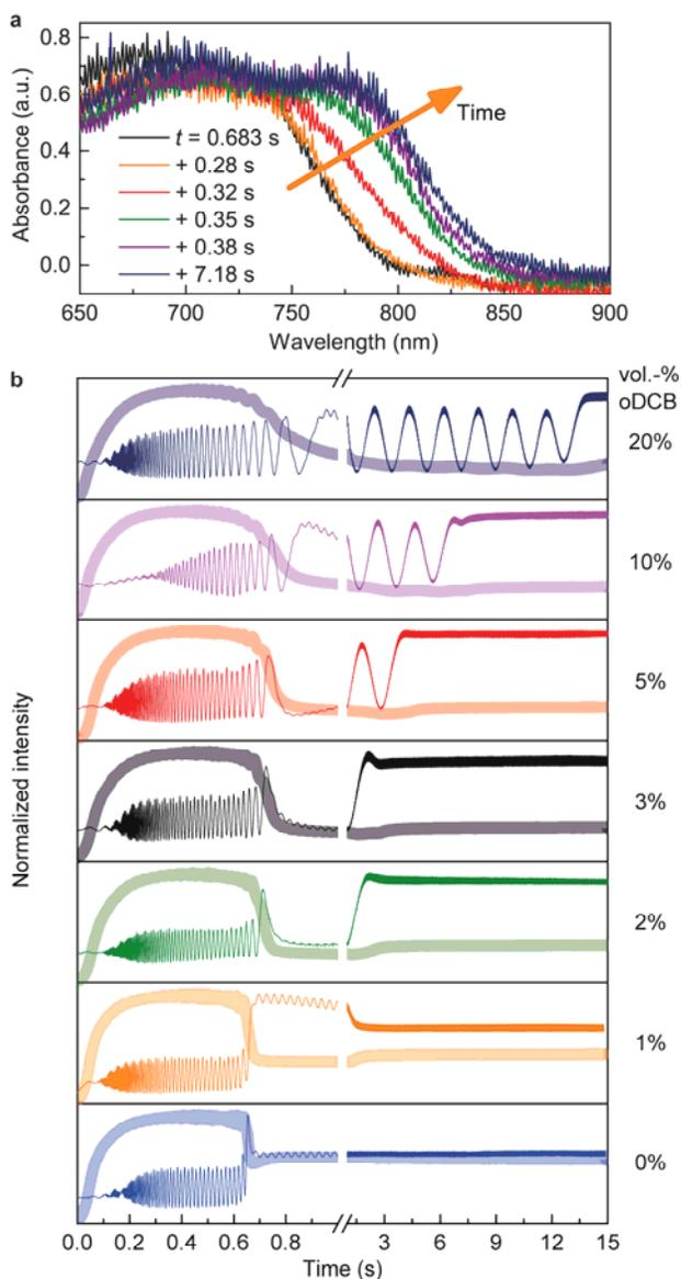
**Figure 4 | Detecting polymer aggregation with time.** **a**, Evolution of the absorption spectrum during spin coating of a PDPP5T:[70]PCBM film from chloroform with 3 vol.-% oDCB. **b**, Laser interference (thin lines) and transmission of 780–820 nm light (thick semi-transparent lines) of PDPP5T:[70]PCBM films during spin coating from chloroform with different concentrations oDCB.
