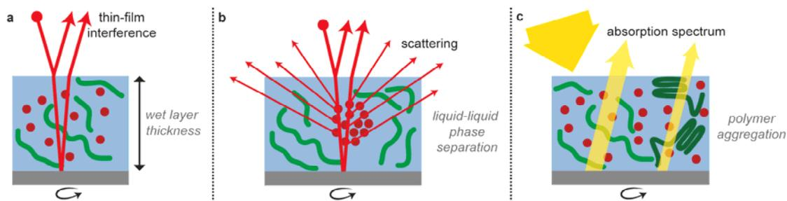
**Figure 2 | Real time optical analysis of film formation.** **a**, The interference of incident laser light is monitored to measure the solvent layer thickness during drying as function of time. **b**, Scattered laser light monitors the onset of liquid-liquid phase separation. **c**, A change in the diffuse reflection of white light detected the change in the absorption spectrum that accompanies aggregation of polymer chains in solution.
