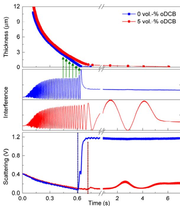
**Figure 3 | Detecting liquid-liquid phase separation with time.** Film thickness, normalized interference, and light scattering of PDPP5T:[70]PCBM in solvent mixtures is monitored during spin coating at 2000 rpm. The solvent is chloroform (blue squares) and chloroform with 5 vol.-% oDCB (red circles). Green arrows schematically indicate the thickness
