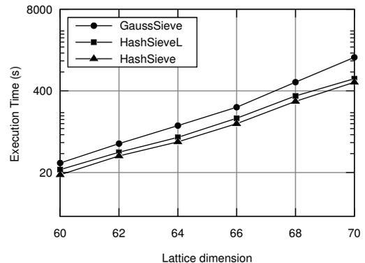
**Figure 2: Execution time, in seconds, for HashSieve with (HashSieveL) and without the probable lock-free system (HashSieve), and GaussSieve (1 thread), on lattices in dimensions 60-70 (less is better).**
