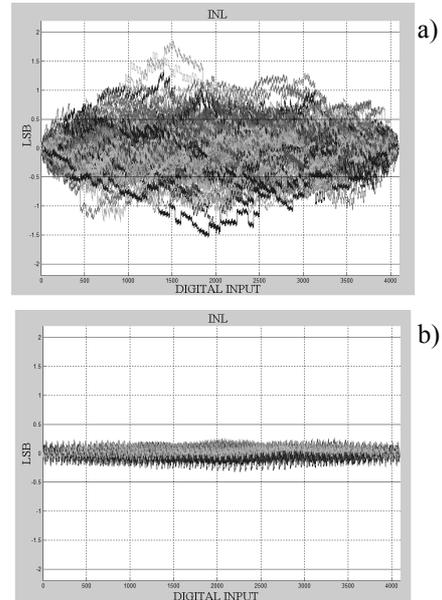
Figure 6: INL for 100 DAC samples: a) pre-calibration (intrinsic); b) post-calibration INL.
