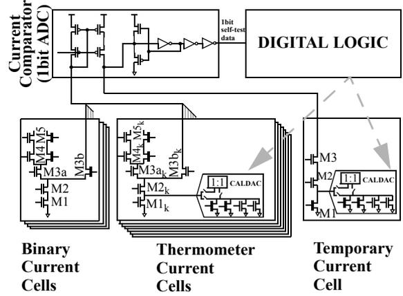
Figure 2: Proposed self-test, self-calibration DAC scheme.
