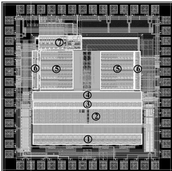
Figure 7: Layout of the 12-bit self-calibrated DAC.
