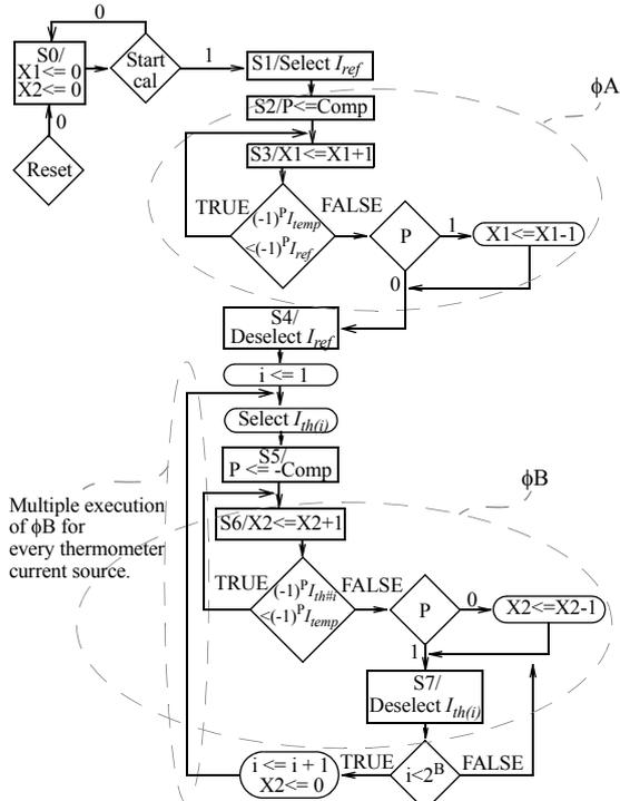
Figure 4: State-Machine chart of the calibration algorithm.
