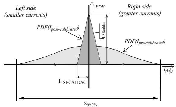
Figure 5: Pre-Calibration and Post-Calibration PDFs.
