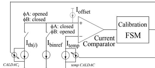
Figure 3: High-level scheme of the proposed calibration algorithm.
