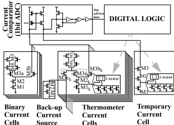
Figure 8: Background calibration variation of the proposed self-test/self-calibration DAC scheme.
