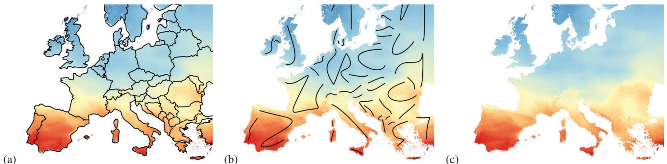
Fig. 17. Solar potential in Europe for horizontally placed PV-modules. Data source: PVGIS 2012.
