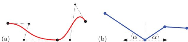
Fig. 4. (a)  $C^1$ -continuous curves have a continuous derivative. The control points of consecutive curves line up. (b) Fixing the required tangent beforehand allows for a dynamic programming solution.
