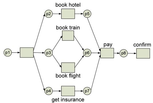
Fig. 12: A system net of a booking process
