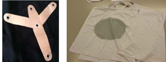
**Figure 2.** (a) The PCB shape in a Kapton polyimide film, attached to fabric using Anorak snaps. (b) Double layer with mesh fabric to adjust the PCB in the Wrap top.
