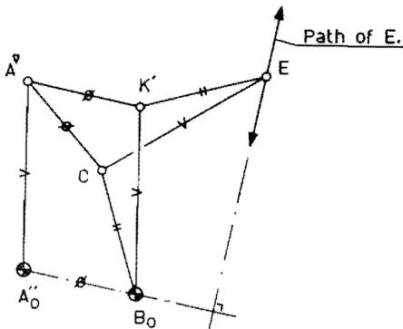
Fig. 11 Straight-line mechanism with 8 bars and 6 turning-joints
