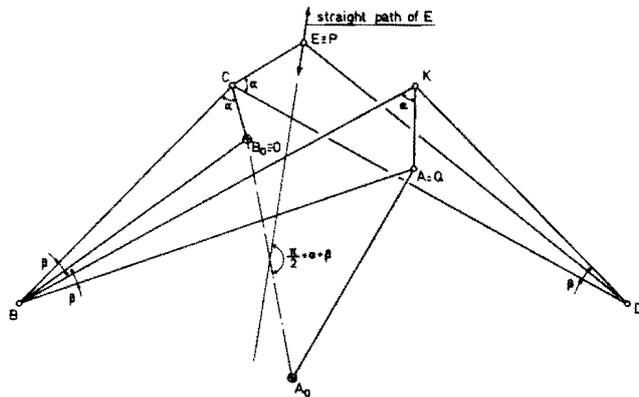
Fig. 3 Quadruplanar inversor of Sylvester and Kempe ( $\overline{OP \cdot OQ} = \text{constant}$ )
