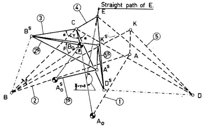
Fig. 4 The quadruplanar inversor of Sylvester and Kempe transformed into another one
