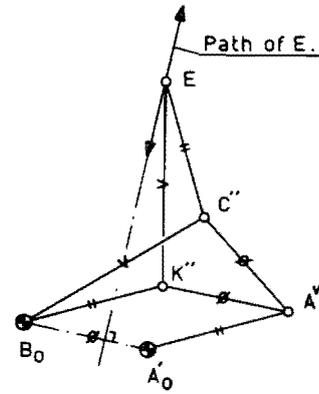
Fig. 15 Straight-line mechanism with 8 bars and 6 turning-joints
