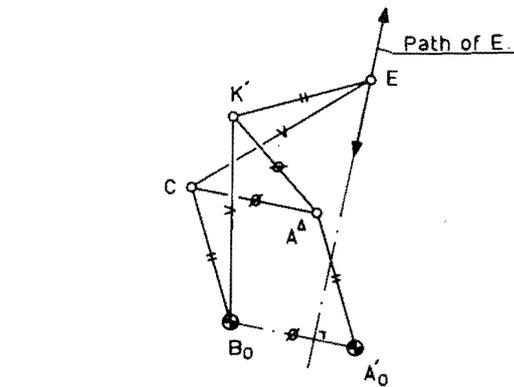
Fig. 12 Straight-line mechanism with 8 bars and 6 turning-joints
