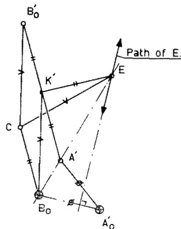
Fig. 9 Invector of the second kind ( $\overline{B_0A'} \cdot \overline{B_0E} = \text{constant}$ )
