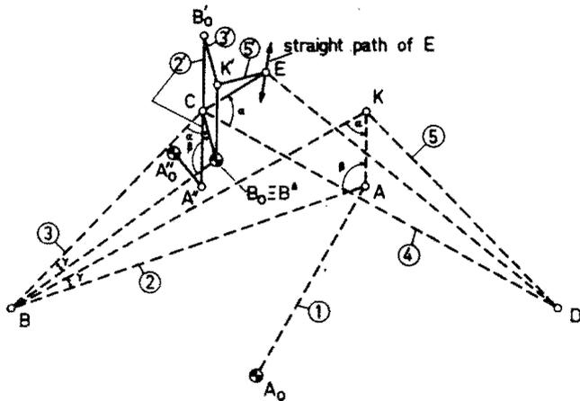
Fig. 6 The quadruplanar invensor of Sylvester and Kempe transformed into a new invensor with 8 links and 7 turning-joints
