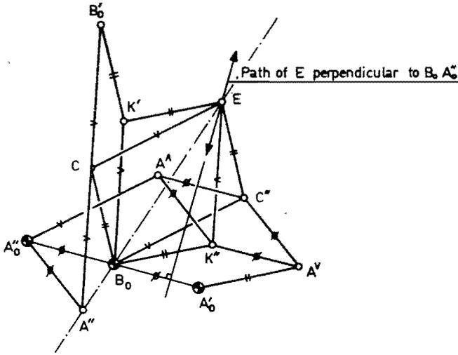
Fig. 13 Second transformation of an invisor into two straight-line mechanisms, both having 8 bars and 6 turning-joints
