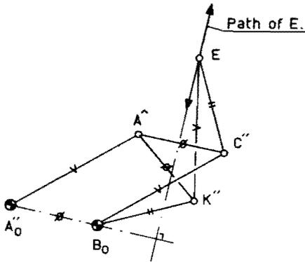
Fig. 14 Straight-line mechanism with 8 bars and 6 turning-joints
