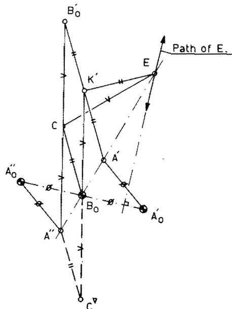
Fig. 8 Two cognate inversion mechanisms of the first and second kind
