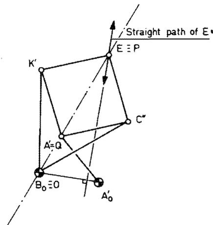
Fig. 1 Inversor of Peaucellier ( $\overline{OP} \cdot \overline{OQ} = \text{constant}$ )
