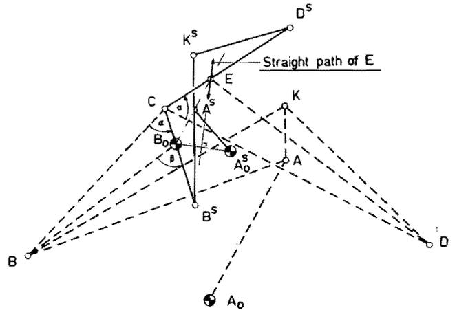
Fig. 5 The quadruplanar inversor of Sylvester and Kempe transformed into the inversor of Hart
