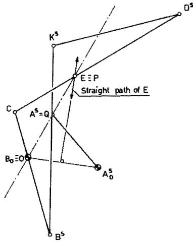
Fig. 2 Inversor of Hart ( $\overline{OP \cdot OQ} = \text{constant}$ )
