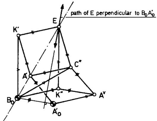
Fig. 16 The invisor of Peaucellier as a cognate of a straight-line linkage
