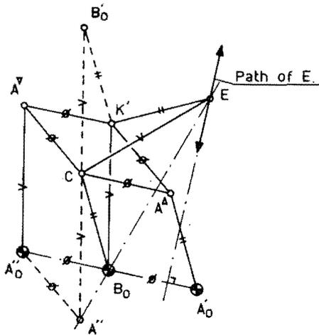
Fig. 10 Transformation of an invensor into two straight-line mechanisms
