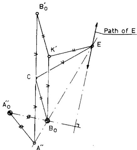
Fig. 7 Invector of the first kind ( $\overline{B_0E} \cdot \overline{B_0A''} = \text{constant}$ )
