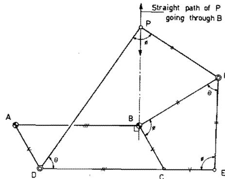
Fig. 17 Planar Kempe linkage of the first kind
