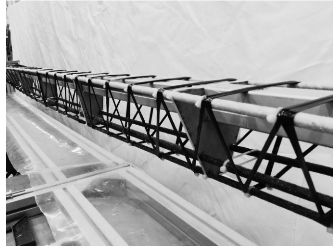
Fig. 20. Bespoke carbon fibre reinforcement for non-prismatic beams; photo: John Orr
