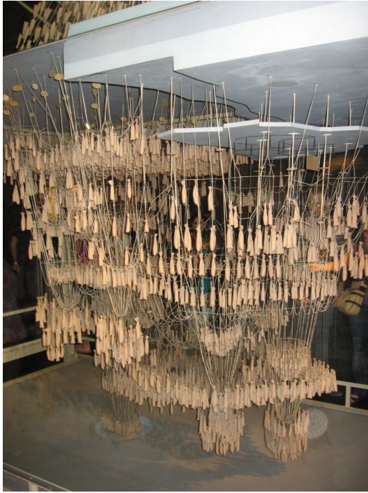
Fig. 10. Recreation of Gaudí's hanging model for the Sagrada Família, Barcelona; photo reproduced under CC-BY-SA/© Canaan [93]
