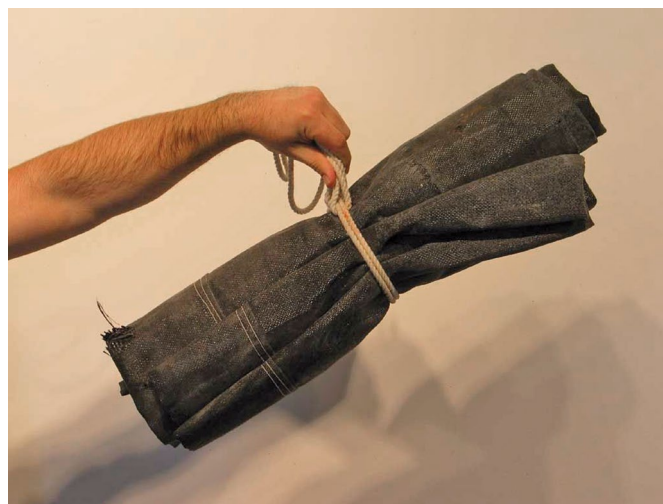
Fig. 18. Easily transportable flexible formwork; photo: Mark West (C.A.S.T.)
