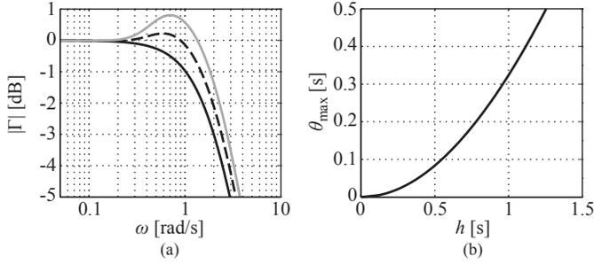
Fig. 3.  $\mathcal{L}_2$  string stability properties: (a) string stability complementary sensitivity magnitude  $|\Gamma(j\omega)|$  for communication delay (solid black)  $\theta = 0$  s, (dashed black)  $\theta = 0.15$  s, (grey)  $\theta = 0.3$  s, and (b) maximum delay  $\theta_{\max}$  as a function of headway  $h$ .
