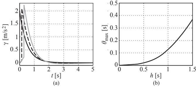
Fig. 4.  $\mathcal{L}_\infty$  string stability properties: (a) impulse response  $\gamma(t)$  for communication delay (solid black)  $\theta = 0$  s, (dashed black)  $\theta = 0.15$  s, (grey)  $\theta = 0.3$  s, and (b) maximum delay  $\theta_{\max}$  as a function of headway  $h$ .
