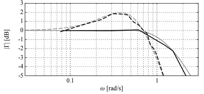
Fig. 5. String stability complementary sensitivity magnitude  $|\Gamma(j\omega)|$ : (solid black) CACC measured, (solid grey) CACC theoretical, (dashed black) ACC measured, (dashed grey) ACC theoretical.
